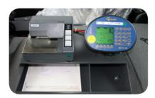
to a receipt. It is also possible to do only a "second" weighing with a full container. The empty container weight can be manually given in by a Preset tare & the net weight can then be calculated.
